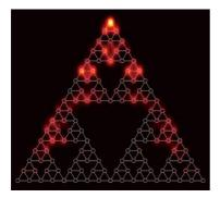
In 2021, we went a step beyond and using photonics experiments we unveiled the quantum dynamics in fractals. By injecting photons in waveguide arrays arranged in a fractal shape, we were able to follow their motion and understand their quantum dynamics with unprecedented detail. We built 3 types of fractal structures to reveal also the influence of geometry [2].
